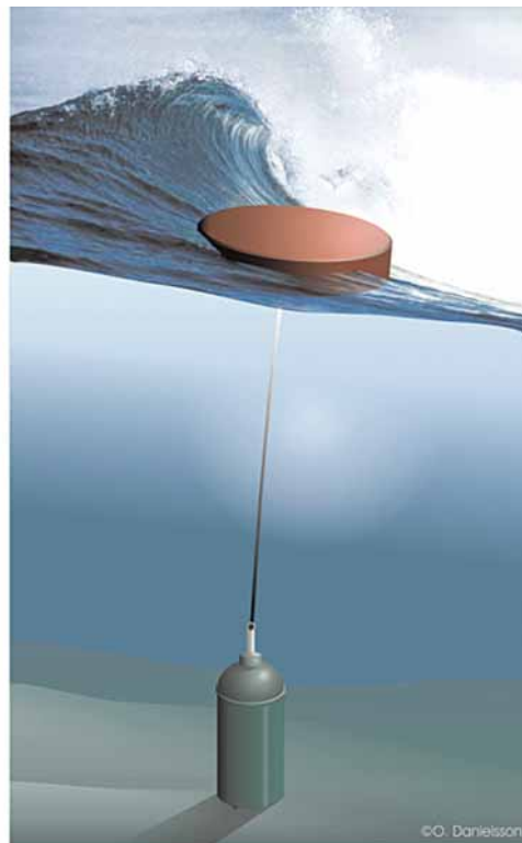
Buoys and point absorbers connected to linear generators. © O. Danielsson
