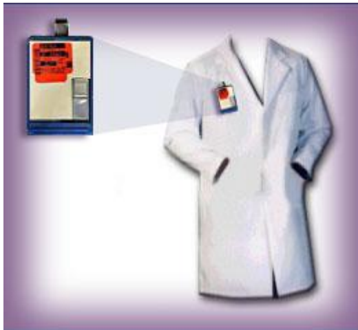
Figure 3.1. Personnel working in an ionizing radiation environment wear dosimeters
