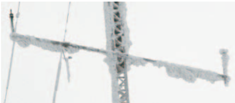
Iced Measurement instruments. Beginning of February at Stor-Rotliden wind farm site.
