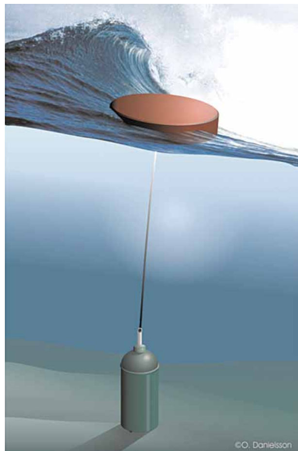
Buoys and point absorbers connected to linear generators. © O. Danielsson
