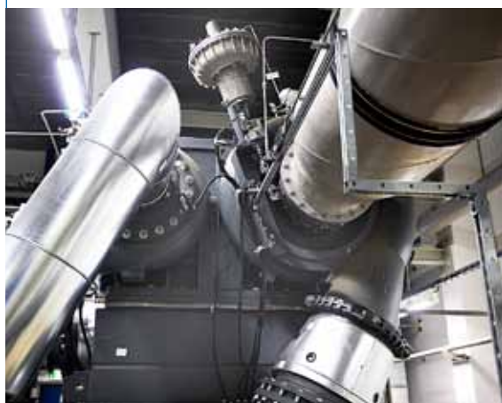
Detail from the CO 2 compression unit in the oxyfuel pilot plant in Schwarze Pumpe
