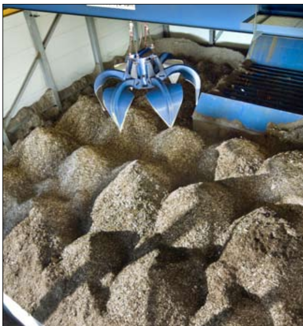
Wood chips fed to the CHP plant in Motala, Sweden
